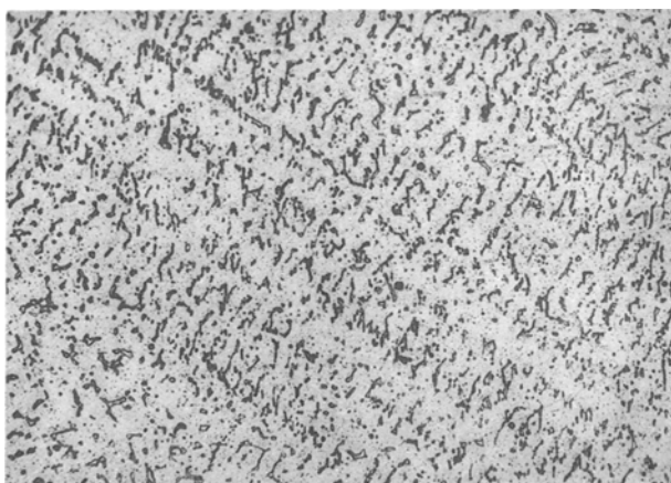
Figure 5 Microstructure of low ferrite sample, 4 FN, PWHT 800 °C, 1 h. × 200.
