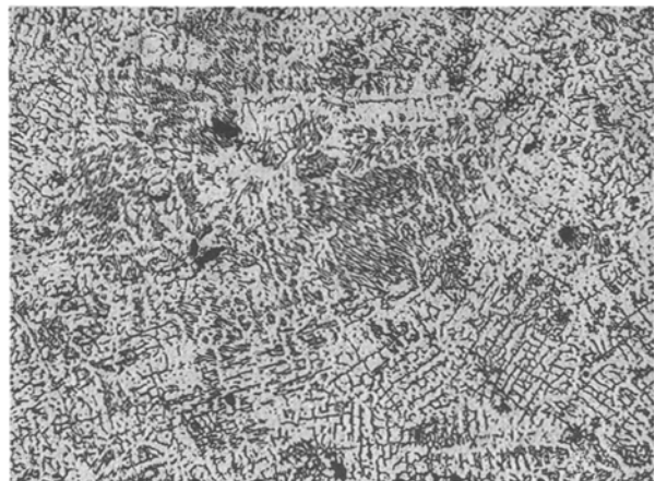
Figure 2 Continuous ferrite morphology in high ferrite (12 FN) sample. × 100.
